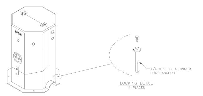
\*Note the receptacles and the concrete slab should be prepared and fully cured before the enclosure is unpackaged.
